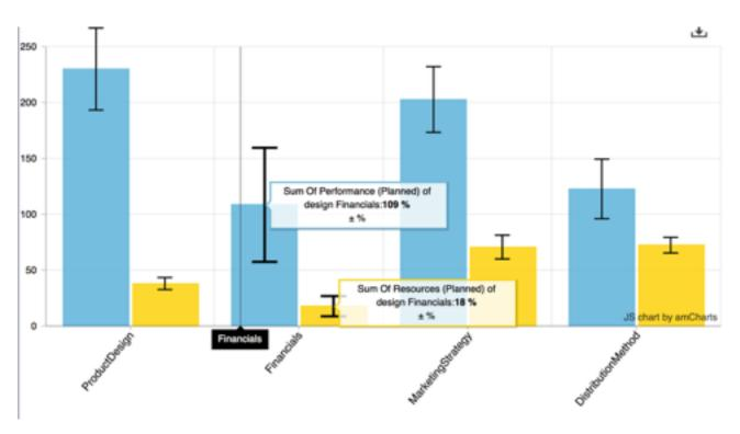
Figure 5 The needs and means tool can provide summaries of the table data such as this. it shows the design options, their total value, their total costs and their uncertainty (the I bars). The tool can sort the options into a prioritized sequence based on efficiency (value to cost), and or by riskiness.
