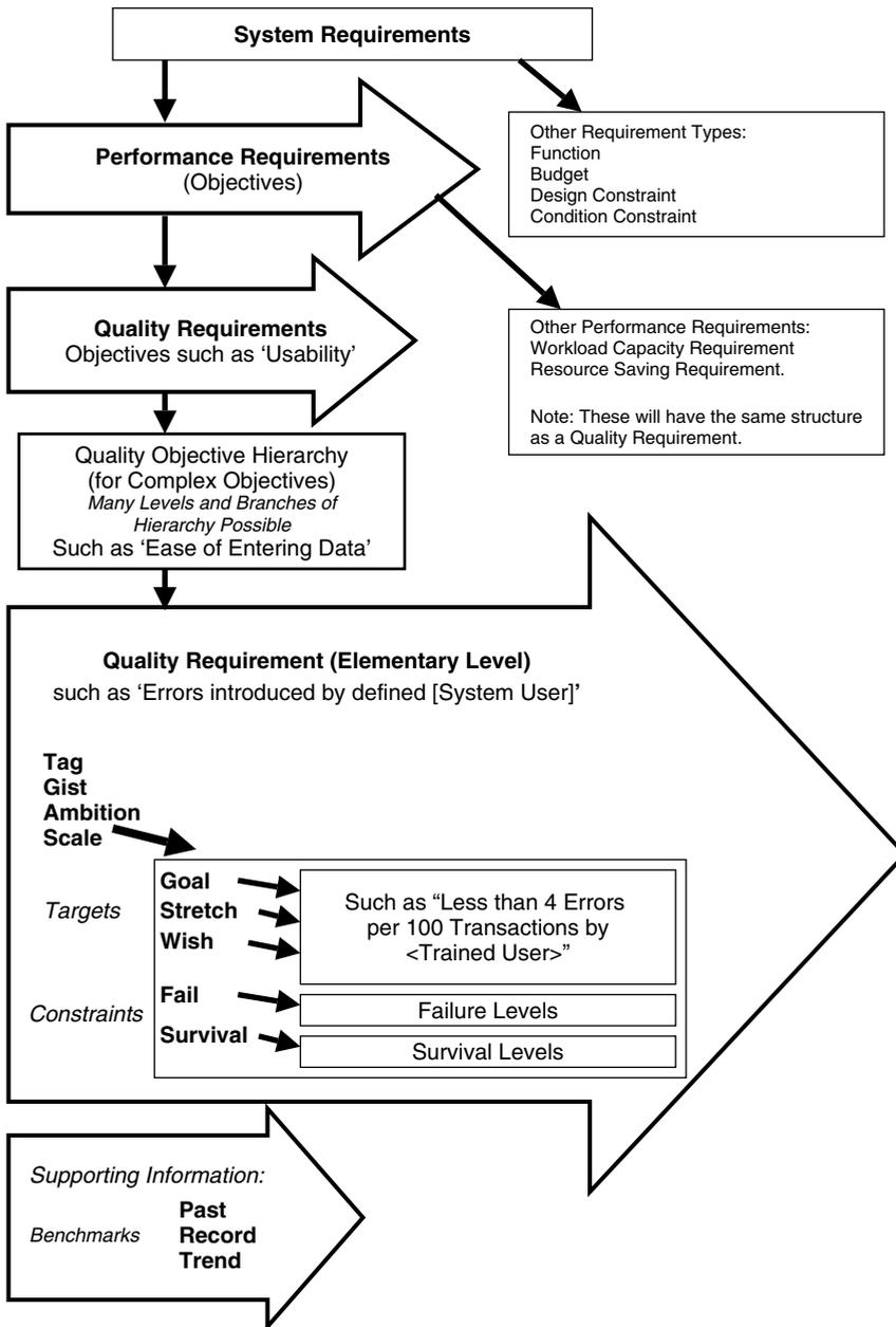
**Figure 4.7** Requirement specification hierarchy for a quality requirement.
