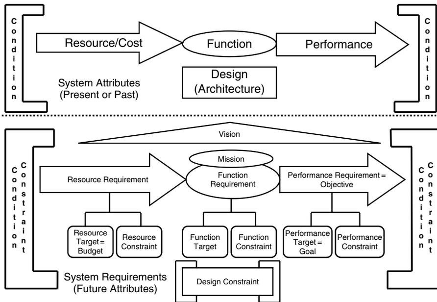
**Figure 2.2** Mapping of system attributes to requirements.
