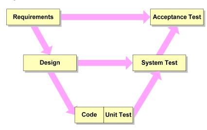
The left side of the "V" represents the specification and construction of software as successive refinements at lower levels of abstraction, in which the outputs of upstream processes are used by their neighbours downstream as sources. The right side represents successive processes of integration and quality assurance (such as testing) at higher levels of abstraction.
